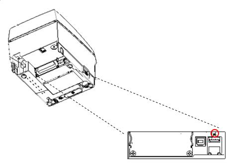
Pressing the Function Key while the power is ON will print the LAN/WLAN setting status page.
