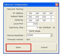
Enter the proper IP Address, Subnet Mask, and Gateway for the currently used network, and then press the Save button to save the settings.
