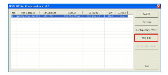
When you press the BSS Info button, information about the SSID, BSSID, Network Model, and Encryption information of the network in close range will be shown as follows.
