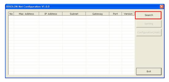
When you press the Search button, the SRP-F310 printer connected to the network will be shown in the list.
