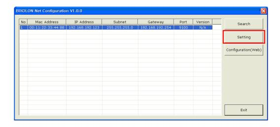
Select the SRP-F310 printer from the list and press the [Setting] button, and then the following window for setting Ethernet settings will pop up.
